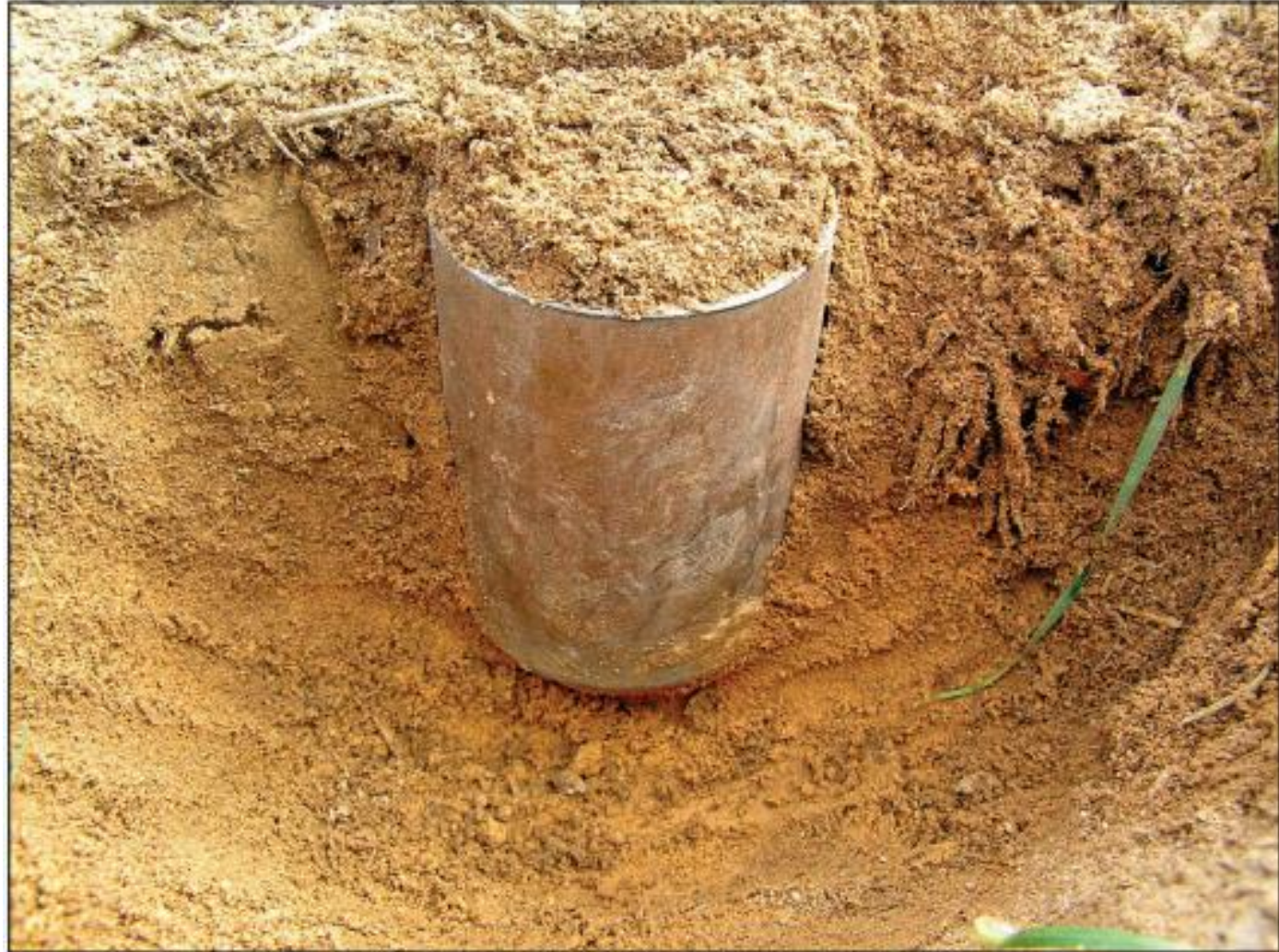
Figure 2: Bulk density ring with intact soil core inside.
